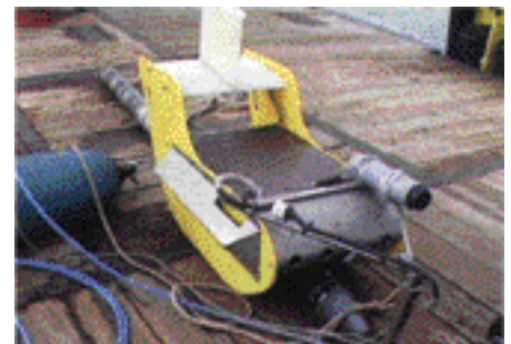
Nn-Shuttle with USBL transponder on its port bow and magnetometer underneath
