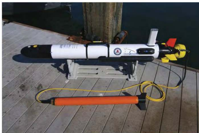
Fig. 1. IVER 2 AUV with EdgeTech 600/1600 kHz side-scan sonar, phase differencing bathymetry system, and an Explorer magnetometer.
